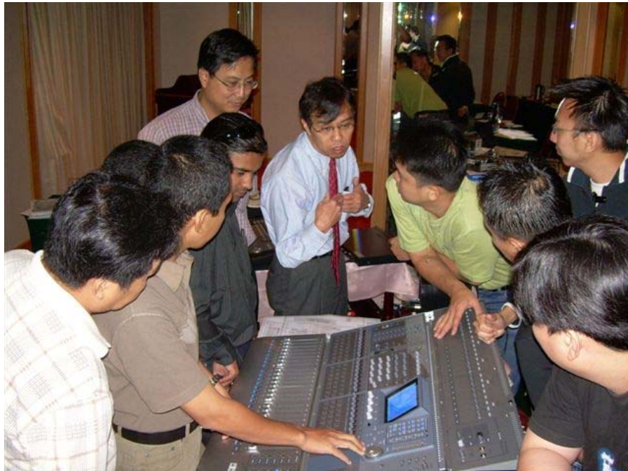
Mr. Takashi Haramoto teaches detailed troubleshooting method on DM-4800, a 64-channel digital mixing console catered to mid-priced broadcast market demand.
